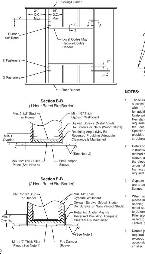
Min. 2-1/2" Runner Min. 2-1/2" Stud Min. 2-1/2" Stud Panhead Screws (Metal Studs) Nails (Wooden Studs) 4 Per 90° Bend
